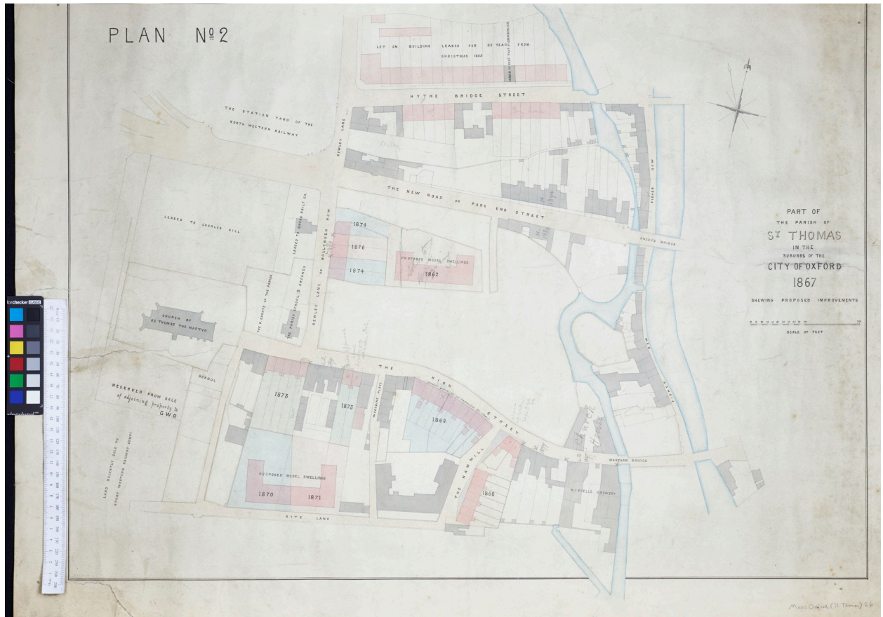
Figure 1. Plan of St Thomas's prepared in 1867 by the Oxford architect, E. G. Bruton, illustrating an ambitious programme for building new housing on the Christ Church estate. Newly-built model dwellings are shown on the corner of The Hamel and Kite Lane, today's Osney Lane. Houses on the east side of The Hamel were built as planned in 1868, but the other dated improvements were never implemented.
